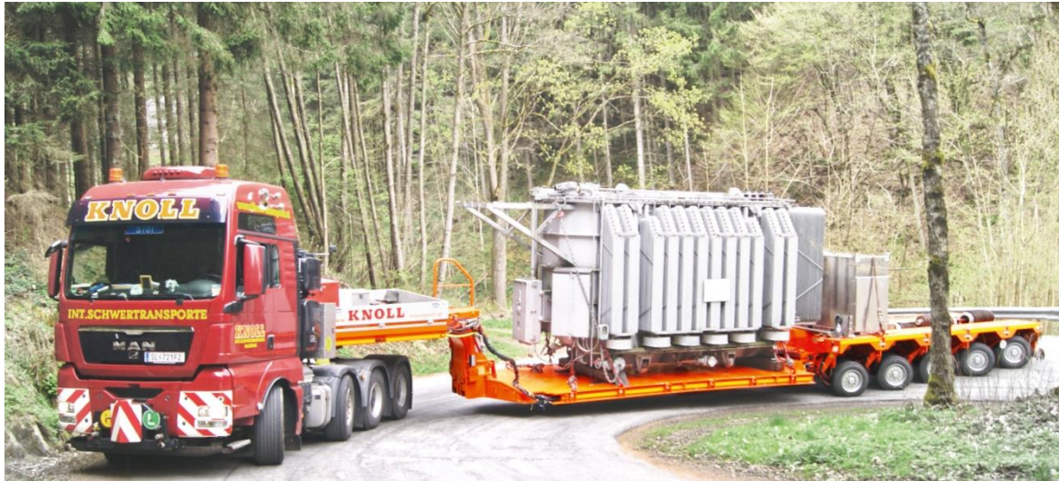
Figure 1-8 Exceptional road transport of a transformer (source: Scheuerle-Nicolas catalogue 35 )
