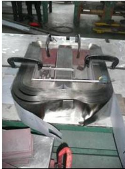
Figure 5-9: Amorphous metal transformer core under construction 119
